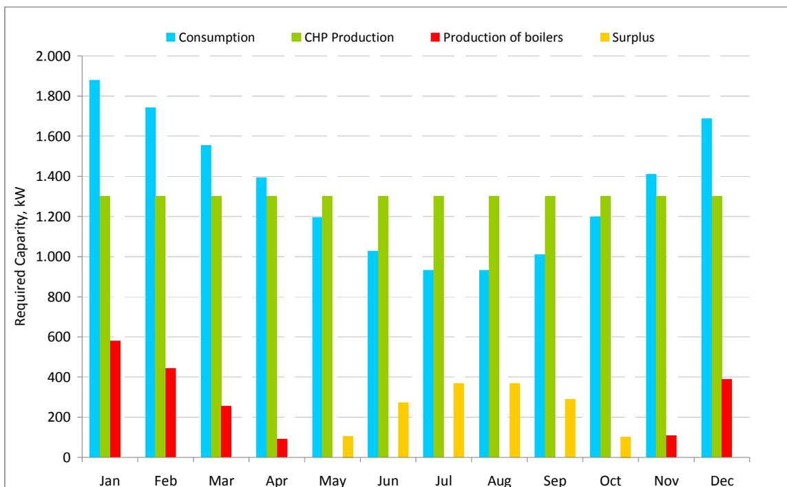
**Figure 3: Possible heat balance for the water treatment plant Buchenhofen**
