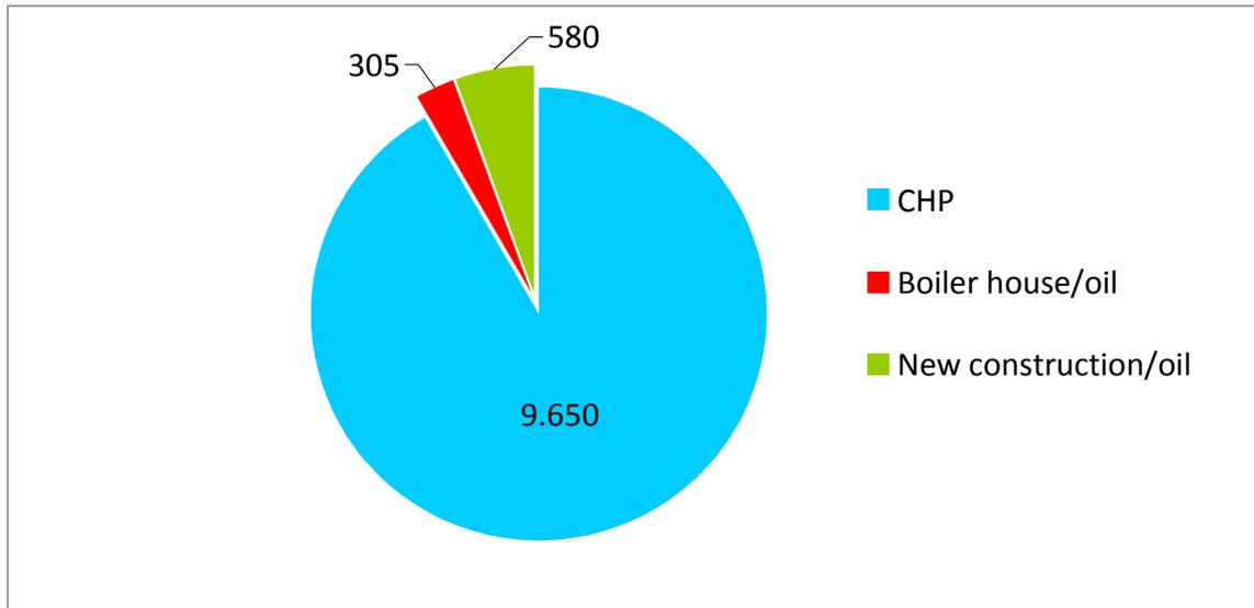
**Figure 2: Distribution of heat production on producers in MWh / a**
