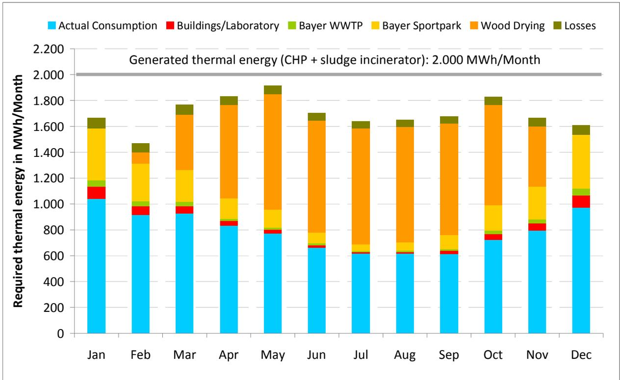
Figure 4: Balance of the thermal energy production of the decentralized heat grid
