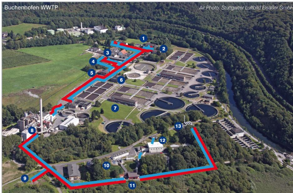
Figure 1: District heating network of the wastewater treatment plant Buchenhofen (The expansion of the network with the laboratory, residential buildings, and the split log drying is already included)
